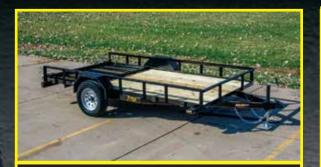
4' Angle Mesh Gate folds flat for transport resulting in increased Fuel Mileage
