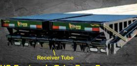
HD Rectangle Tube Rear Bumper w Flush Mount, Fully Sealed Lifetime LED Lights 6" Channel Side Rails
